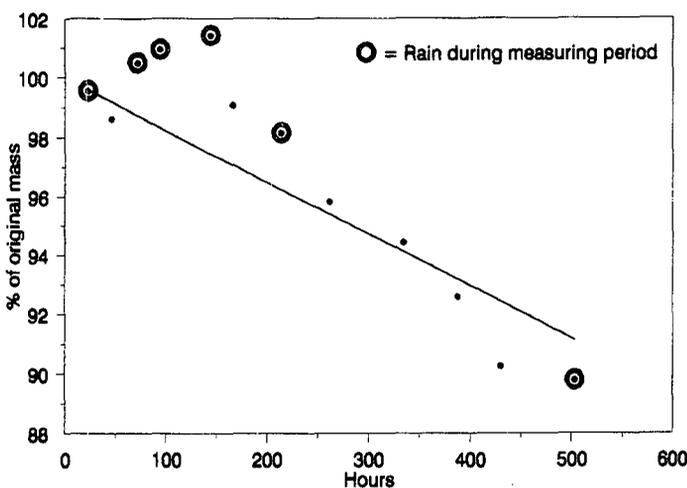
FIGURE 2 Mass loss from a four ton bundle
