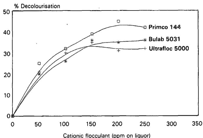
**FIGURE 2** Effect of dosage levels of Primco 144, Bulab 5031 and Ultrafloc 5000 on decolourisation.
