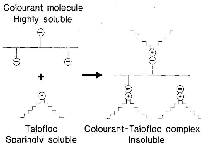
FIGURE 1 Mode of interaction of Talofloc with colourant.
