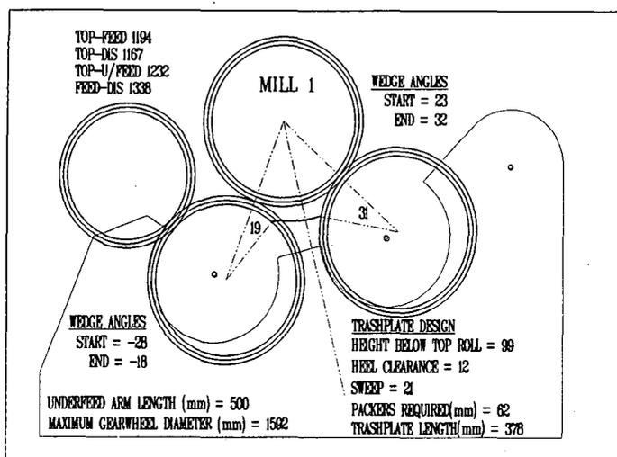
FIGURE 7 Design and information produced by the CAD trashplate design.
