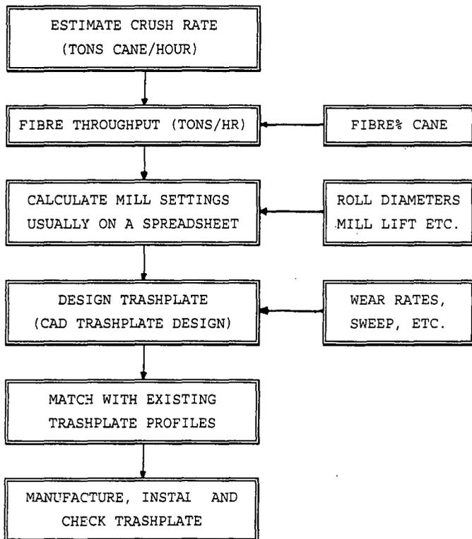
FIGURE 4 Mill and trashplate design flow diagram.
