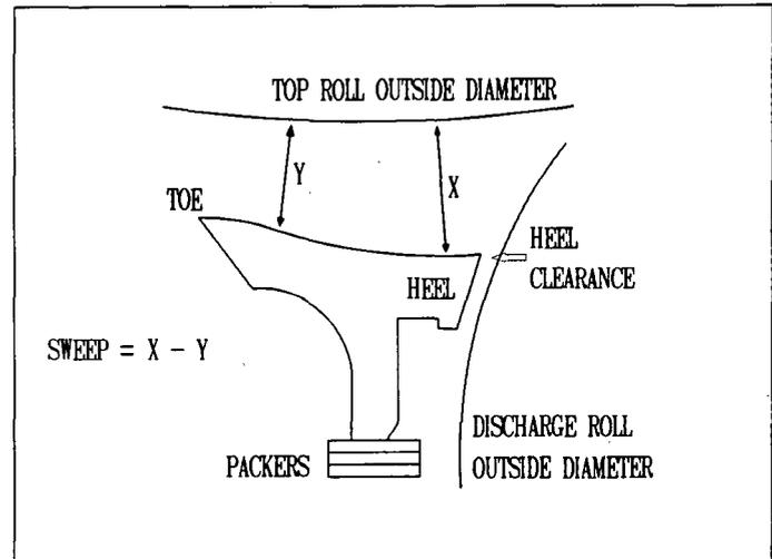
FIGURE 2 A mill trashplate.
