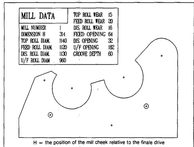
FIGURE 6 Information required for the CAD trashplate design.
