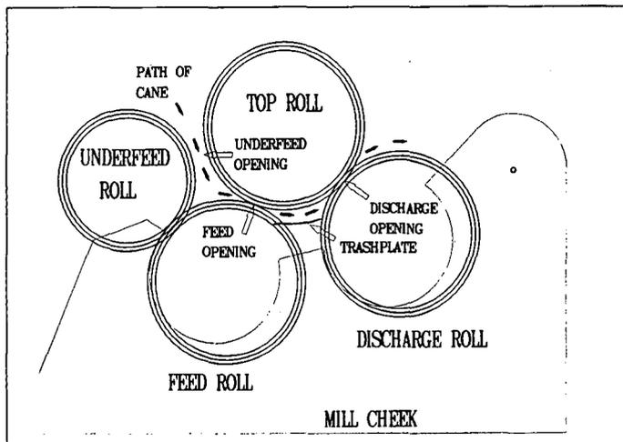
FIGURE 1 General arrangement of a Noodsberg mill.
