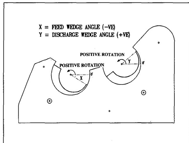
FIGURE 3 Mill wedge arrangement.
