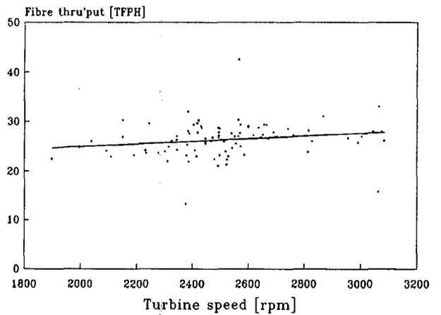
FIGURE 9 Fibre throughput versus turbine speed
