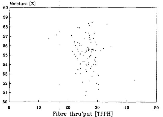
FIGURE 8 Moisture versus fibre throughput
