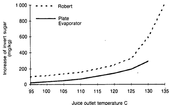
FIGURE 6 Comparison of inversion in different evaporators at different temperatures (Licha et al., 1989).
