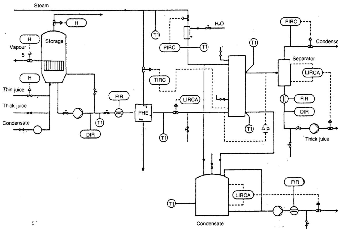
FIGURE 1 Sketch of the pilot plant at the Waghausel factory of Sudzucker AG.
