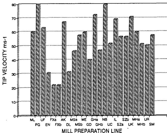
FIGURE 2 Distribution of the tip velocity of knives
