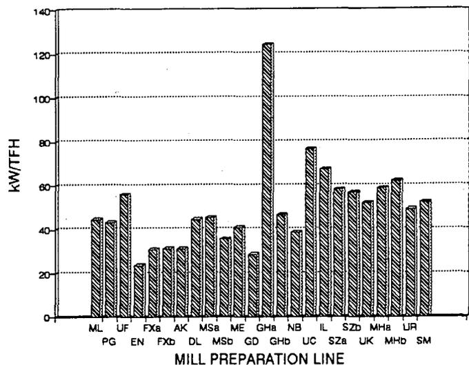
FIGURE 1 Distribution of specific power consumption of knives
