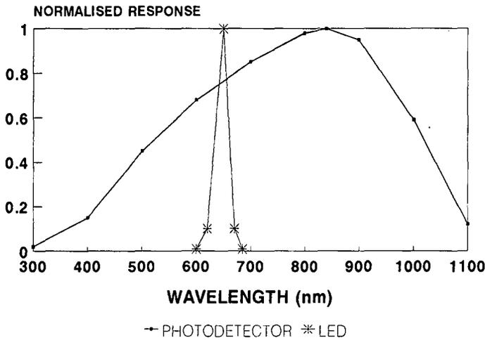
FIGURE 2 Spectral response of photodetector and LED.
