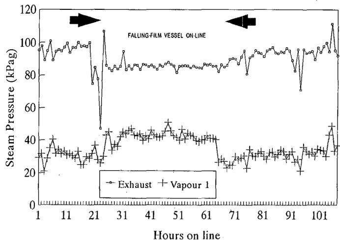
FIGURE 3 Impact of additional area on pressure ranges.
