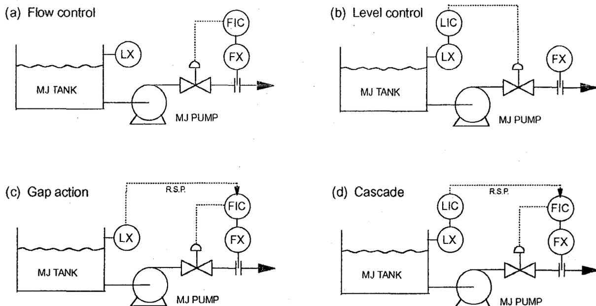
**FIGURE 2:** Standard mixed juice flow control schemes
