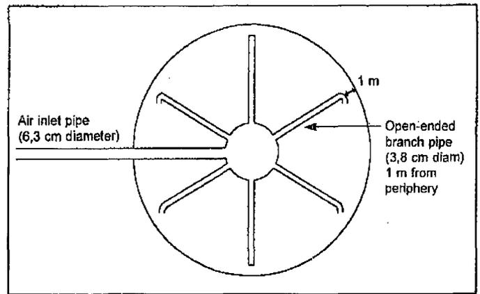
**FIGURE 1:** Top view of the air injection system 20 cm above the base of a molasses storage tank
