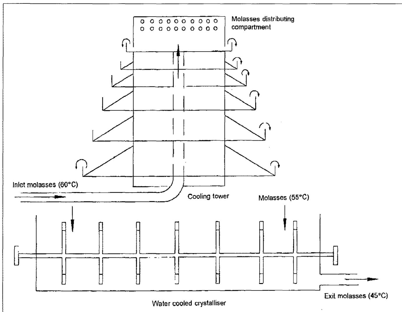
FIGURE 2: Molasses cooling system at FUEL factory after modification
