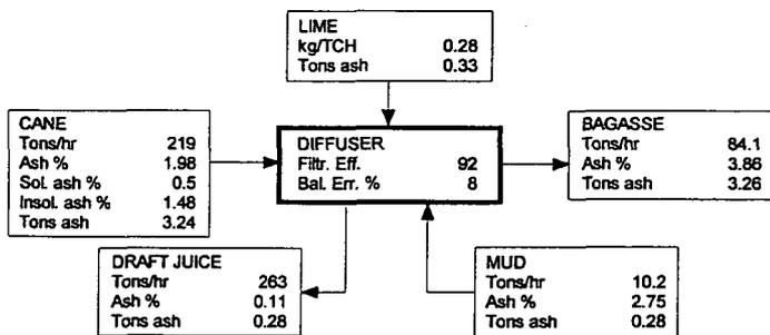
Figure 5. Ash mass balance for Trial 2.
