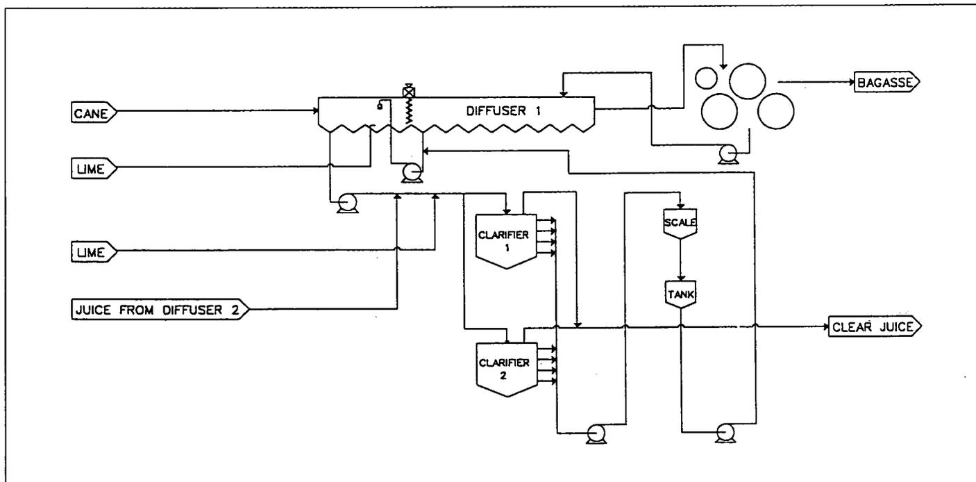
Figure 1: Process flow diagram of mud recycle.
