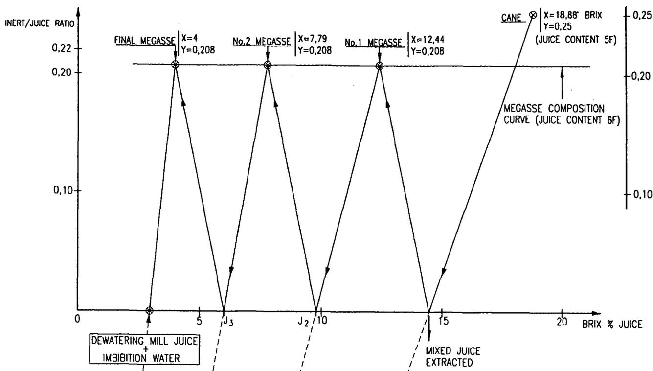
Figure 3. Ponchon-Savarit diagram for number of stages needed for displacement process.
