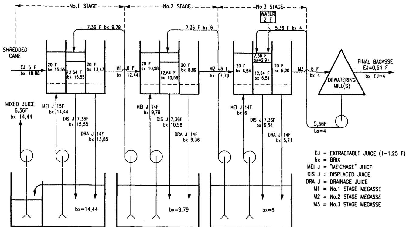
Figure 4. Flow diagram for Rivière juice extractor.
