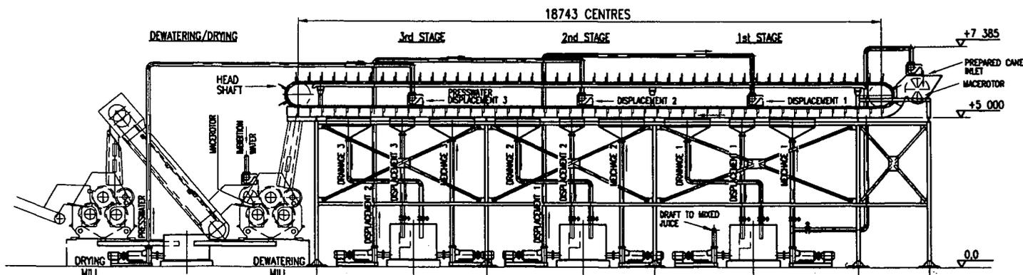
Figure 5. Rivière juice extractor – plant layout.
