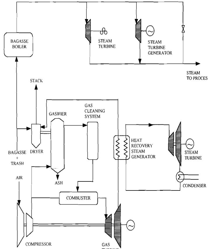
Figure 2. BIG-CC - mill basic integration modes (independent mode).
