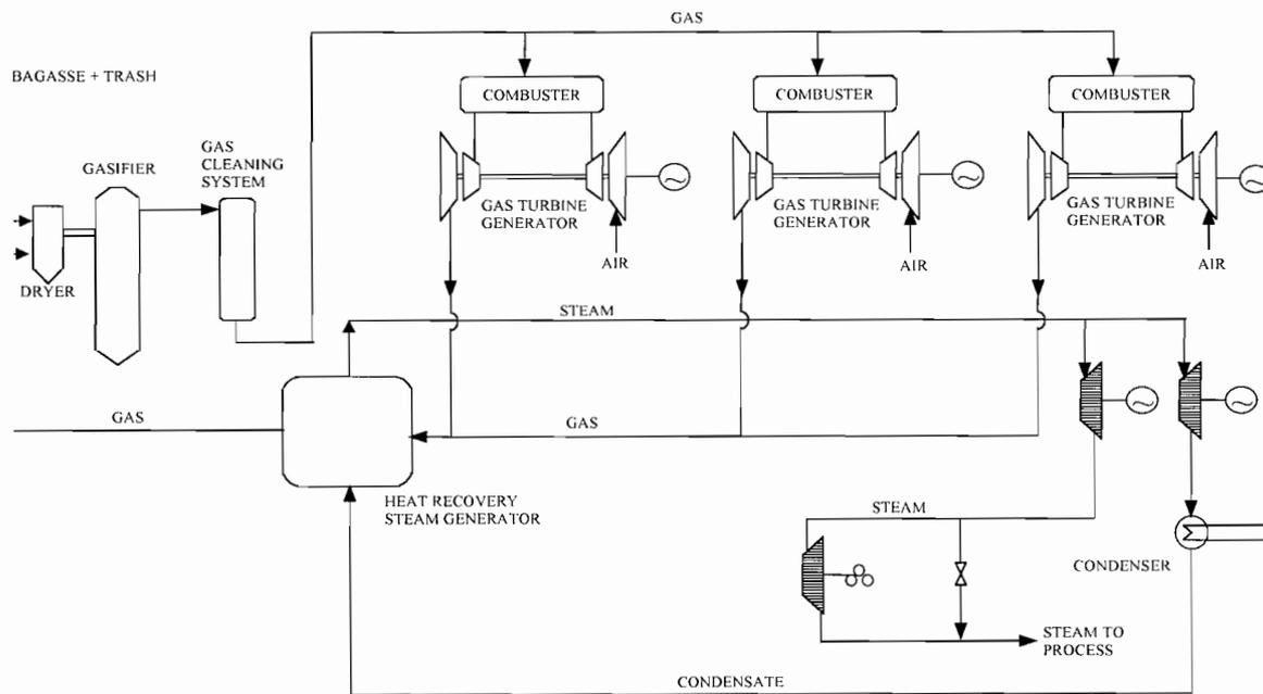
Figure 3. BIG-GT – mill basic integration mode (cogeneration mode).
