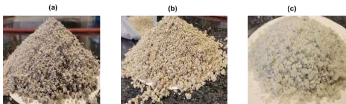
Figure 5. The visual appearance of K 2 SO 4 crystals after different purification processes (a) crystals from first crystallisation, (b) second crystallised crystals, and (c) decolourised crystals
