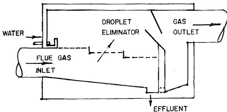
FIGURE 2 Perforated plate scrubber in brick housing.
