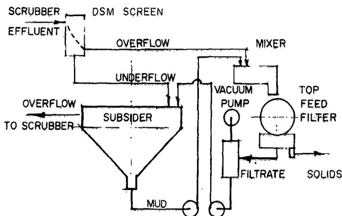
FIGURE 4 Subsider and filter.
