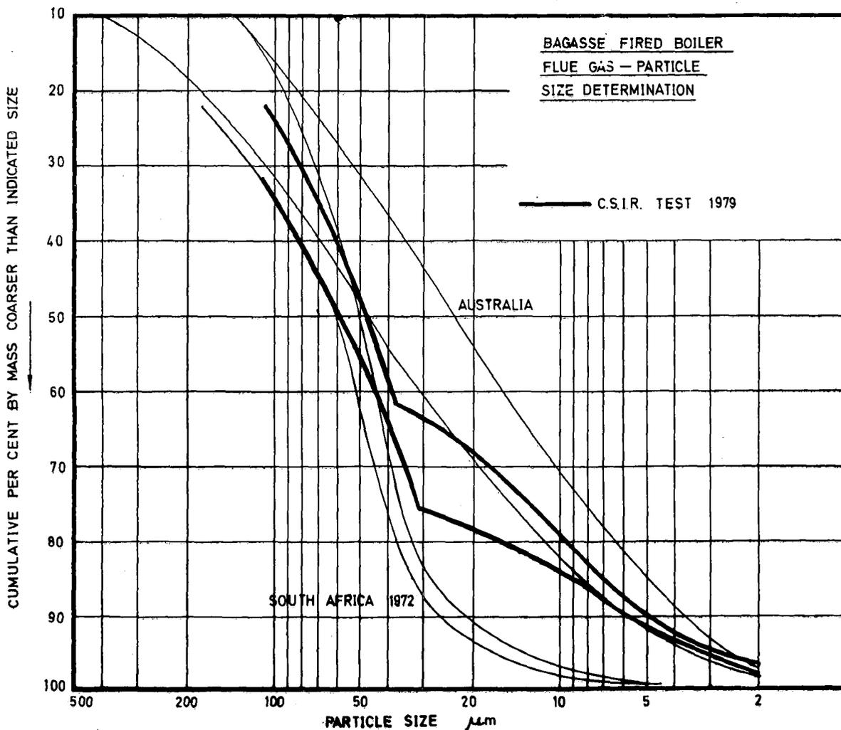
FIGURE 5 CSIR Flue Gas particle size determination.
