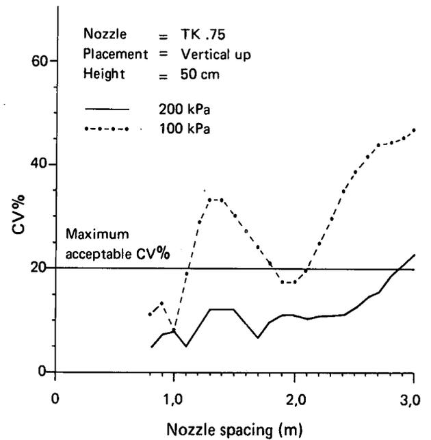
**FIGURE 2** Effect of pressure on range of acceptable nozzle spacings.
