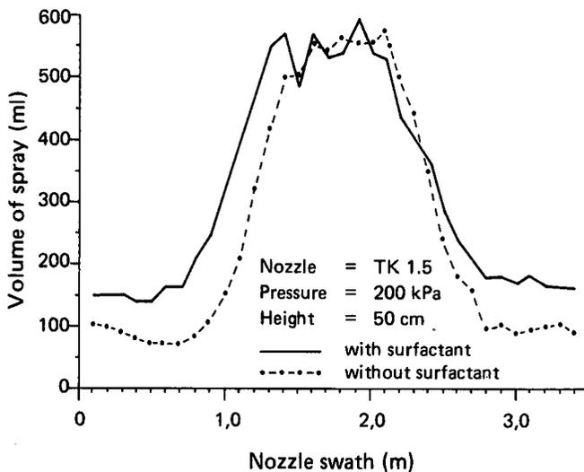
**FIGURE 1** Effect of surfactant on spray distribution pattern.
