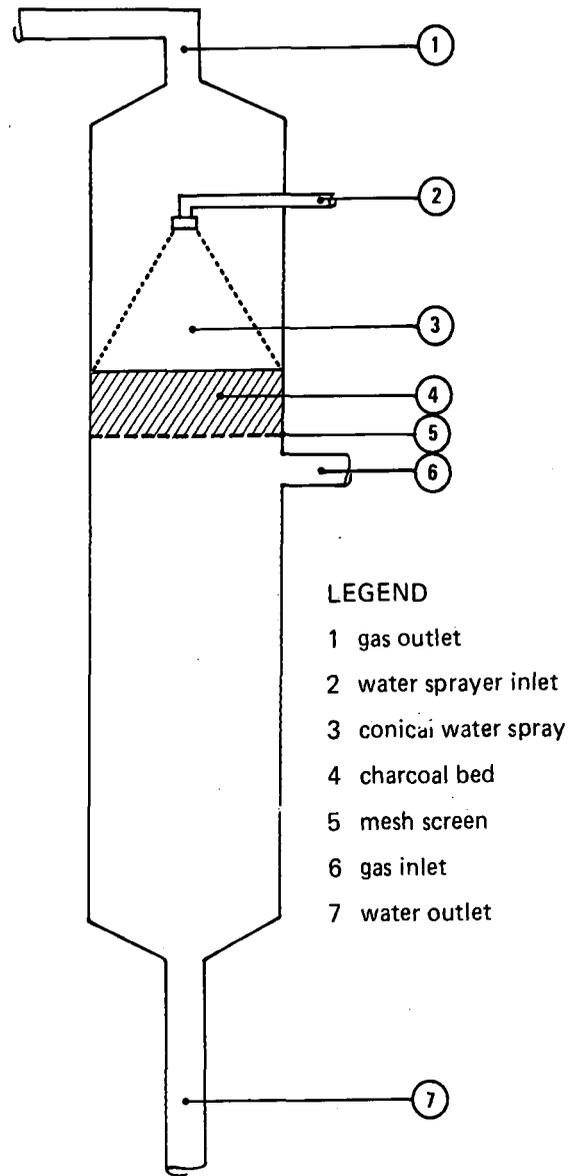
FIGURE 5 Diagram showing section of water scrubbers.
