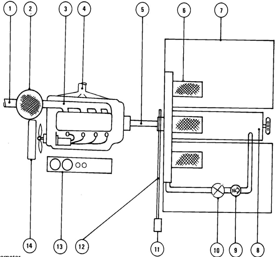
**FIGURE 6** Schematic plan view of engine and dynamometer.
