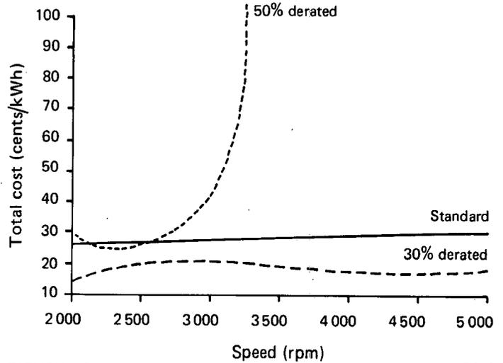
FIGURE 10 Total cost versus speed for 3 levels of derating: 50%, 30% and standard - gas and diesel.
