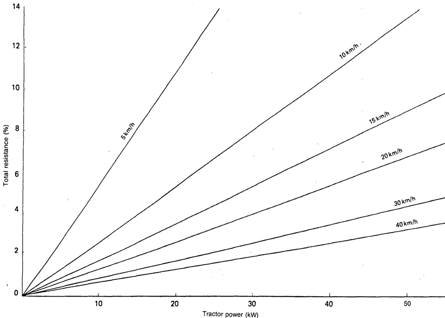
FIGURE 1 Tractor power required (GCM: 10 800 km)
