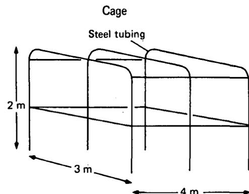
FIGURE 4 Large cage used for releasing *T. applanatus*.
