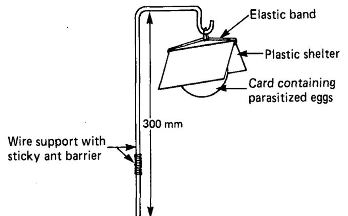
FIGURE 3 Plastic shelter on wire support for mass release of egg parasitoids.
