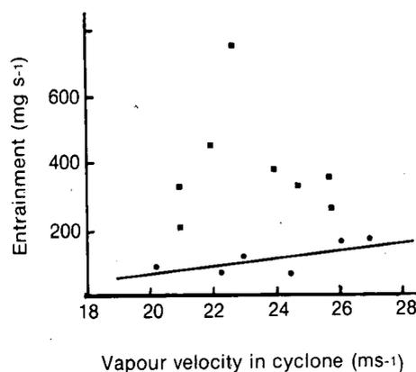
FIGURE 2 Entrainment in an A-pan
