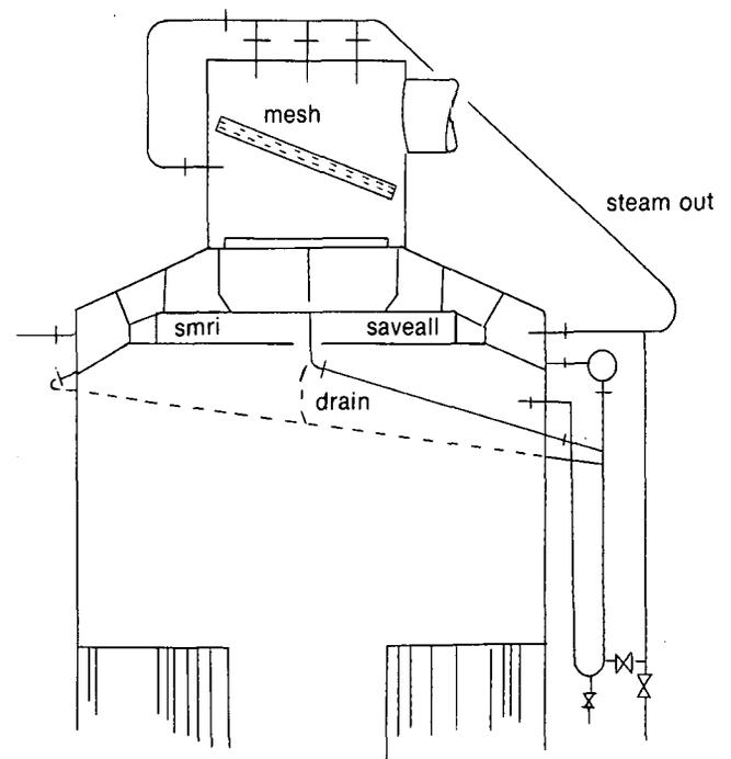
FIGURE 4 Proposed arrangement for draining and steaming out the pan separator
