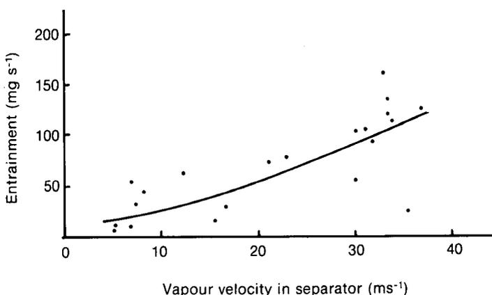
FIGURE 3 Entrainment from a C-pan with a top-hat separator
