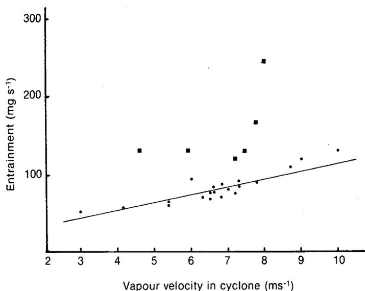
FIGURE 1 Entrainment in mg of sugar per second against vapour velocity for a cyclone separator
