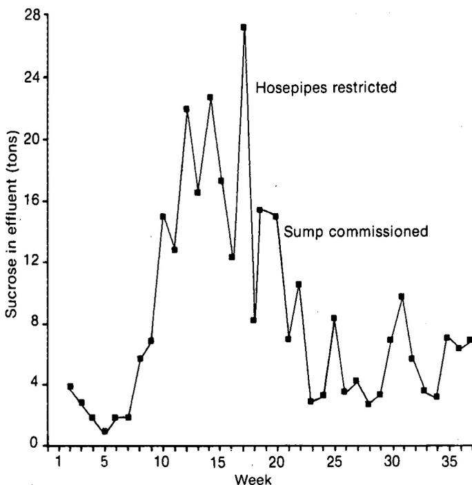
FIGURE 6 Weekly losses in effluent in the 1982-83 season
