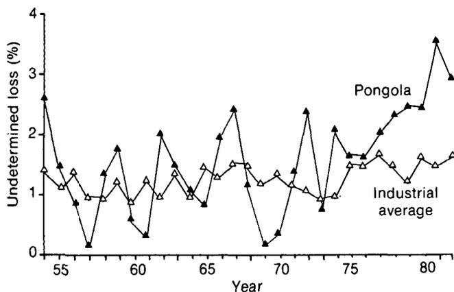
FIGURE 1 Annual undetermined losses for Pongola and industrial average. (Data are based on pol. Prior to 1976 sucrose in molasses was determined by Lane and Eynon, whilst before 1972 sucrose in mixed juice was by Jackson and Gillis).
