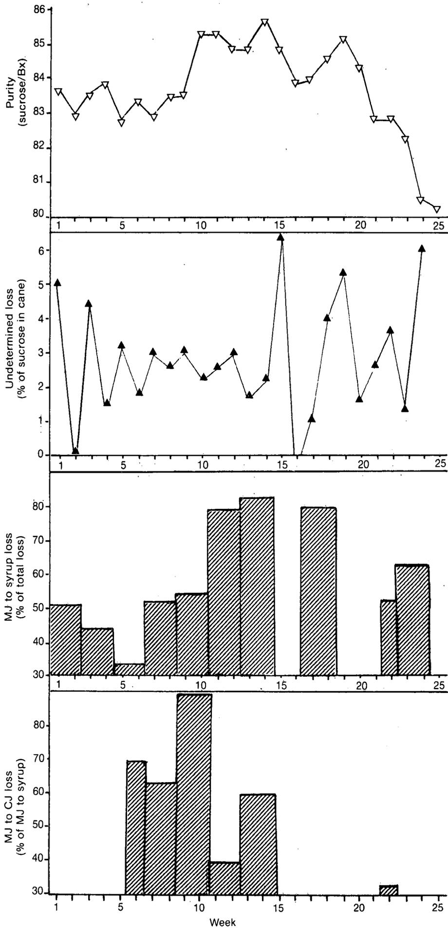
FIGURE 9 Weekly mixed juice purity, undetermined loss, mixed juice-to-syrup loss and mixed juice-to-clear juice loss for the 1983-84 season
