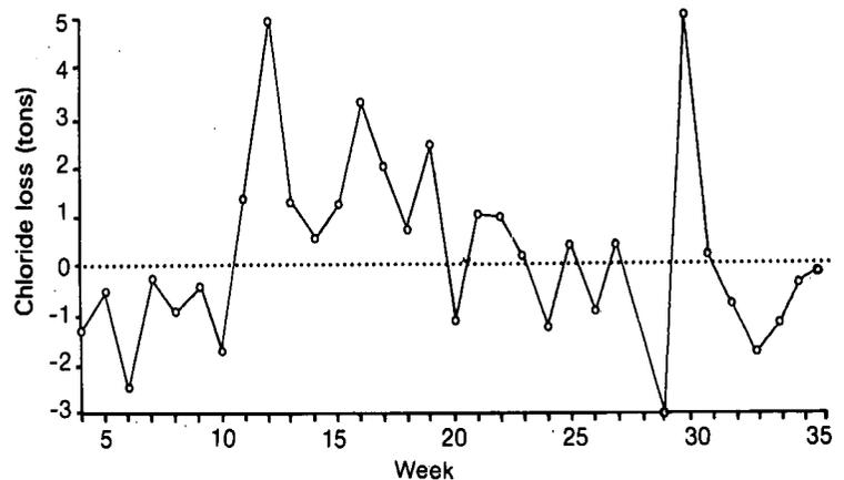
FIGURE 7 Weekly chloride balance between syrup and molasses
