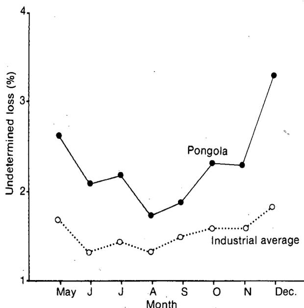
FIGURE 5 Seven-year (1975-81) mean undetermined losses for different months
