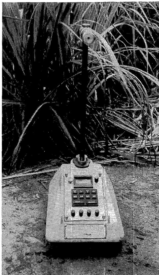
FIGURE 1 Troxler nuclear density and moisture gauge.
