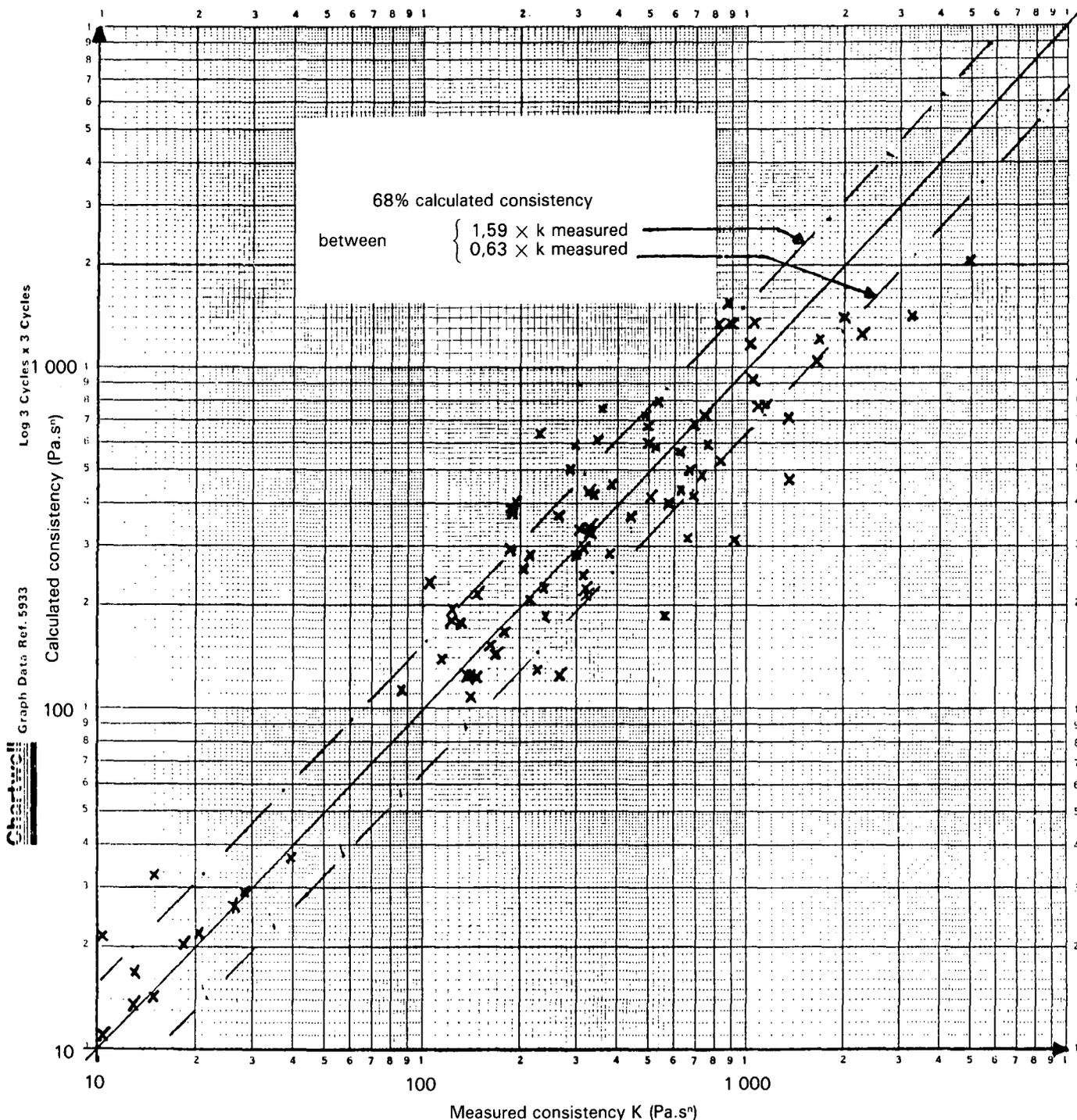
FIGURE 5 Calculated consistency versus measured consistency samples C-masseccuite and C-nutsch.
