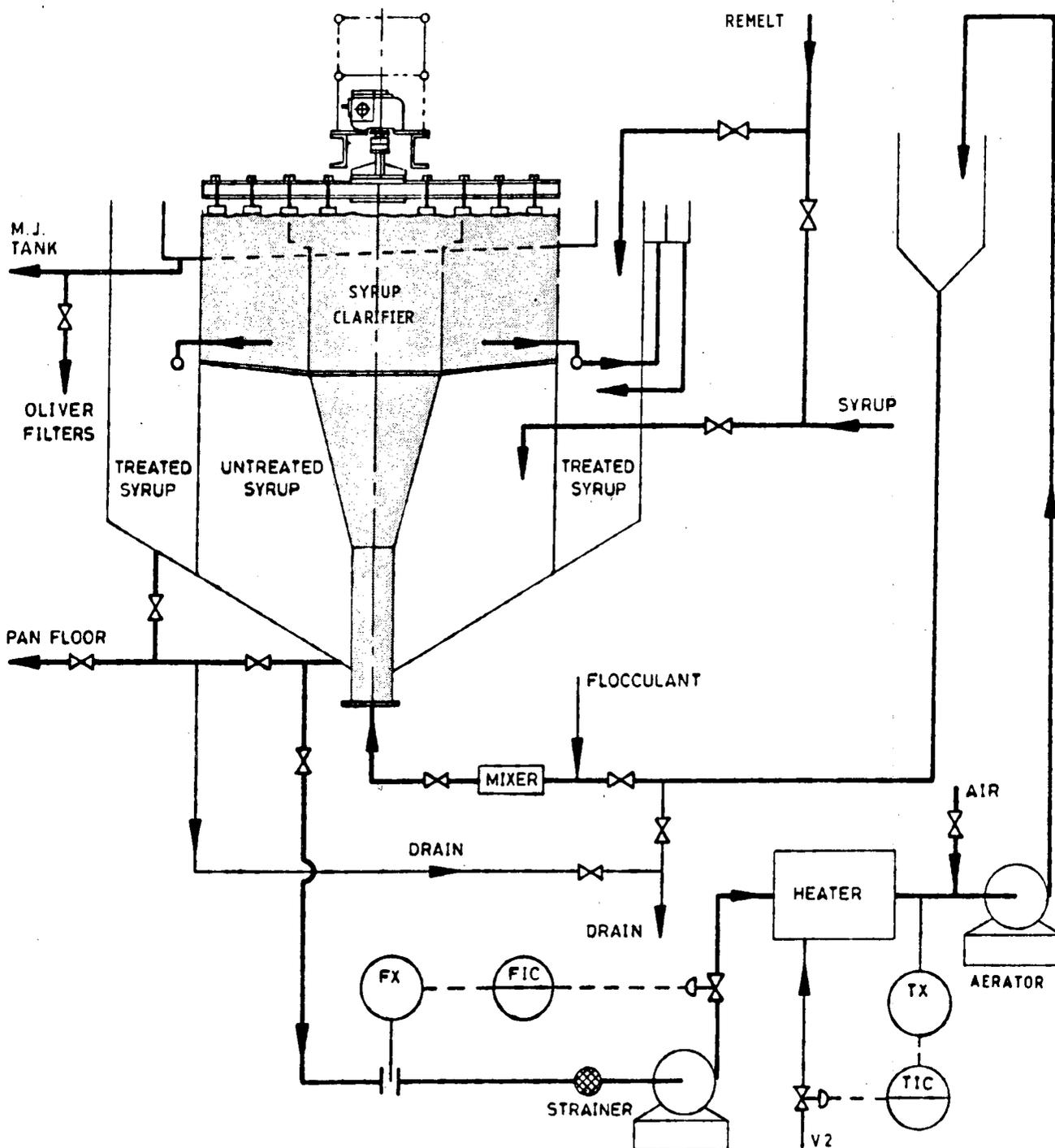
FIGURE 5 Flow diagram for Empangeni syrup clarification.
