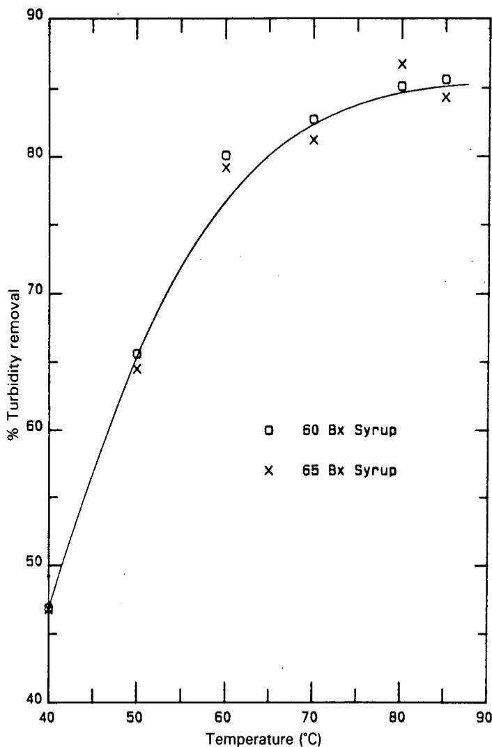
**FIGURE 2** Effect of temperature on turbidity removal.
