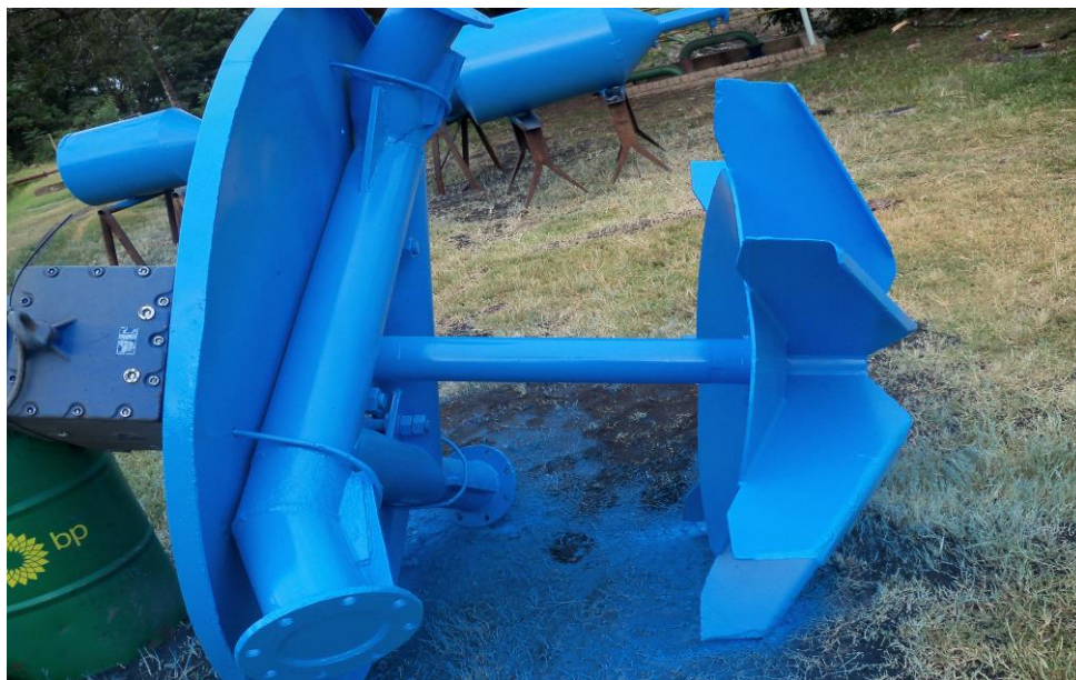
Figure 11. Refurbished aerator from the aeration pond.
