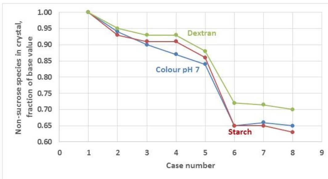
Figure 9: The effect of different crystallisation schemes on the quality of the sugar (No specific properties given for dextran)
