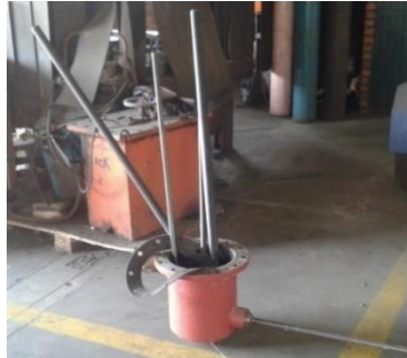
Figure 9. Pipeline viscometer after fabrication with pipelines
