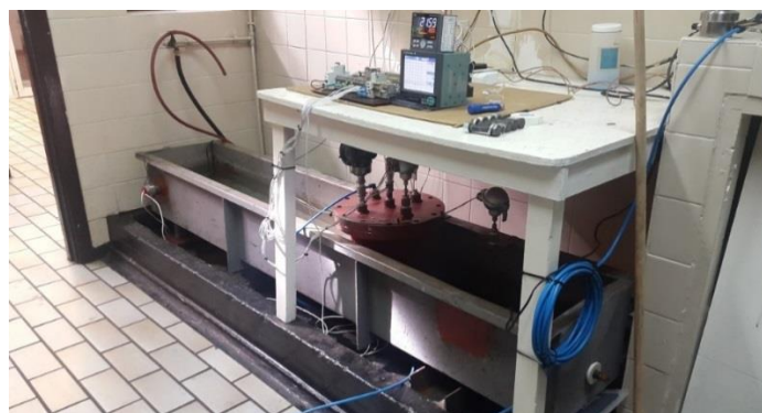
Figure 8. Pipeline viscometer in the waterbath
