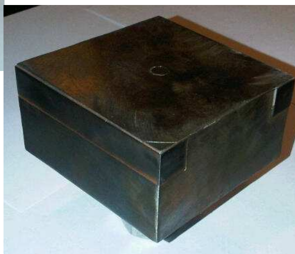
Figure 5. The IMCO sintered tungsten carbide block.
