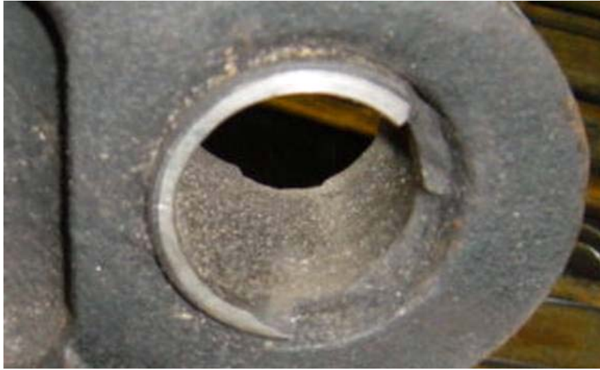
Figure 2. Worn Ausrex inner link.
