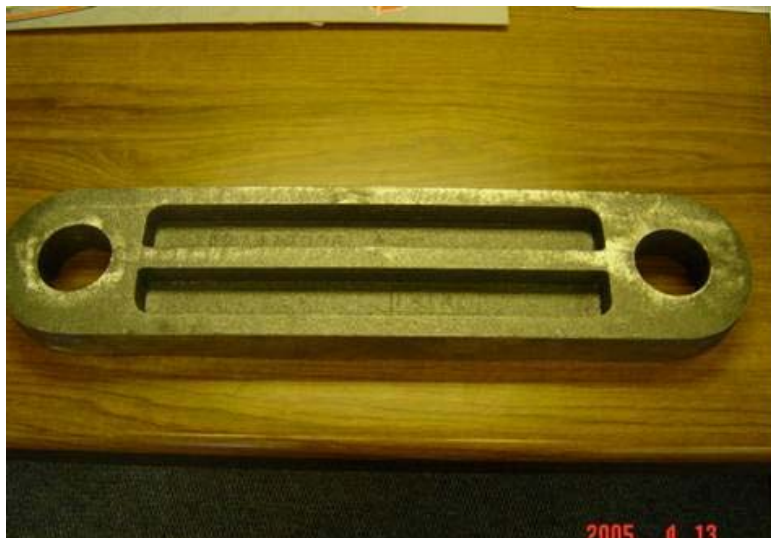
Figure 3. Experimental side link with added centre stiffener.
