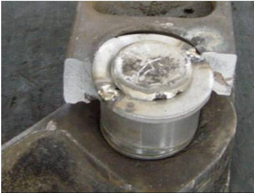
Figure 10. Failed test sample B1-B2-L1-L2.
