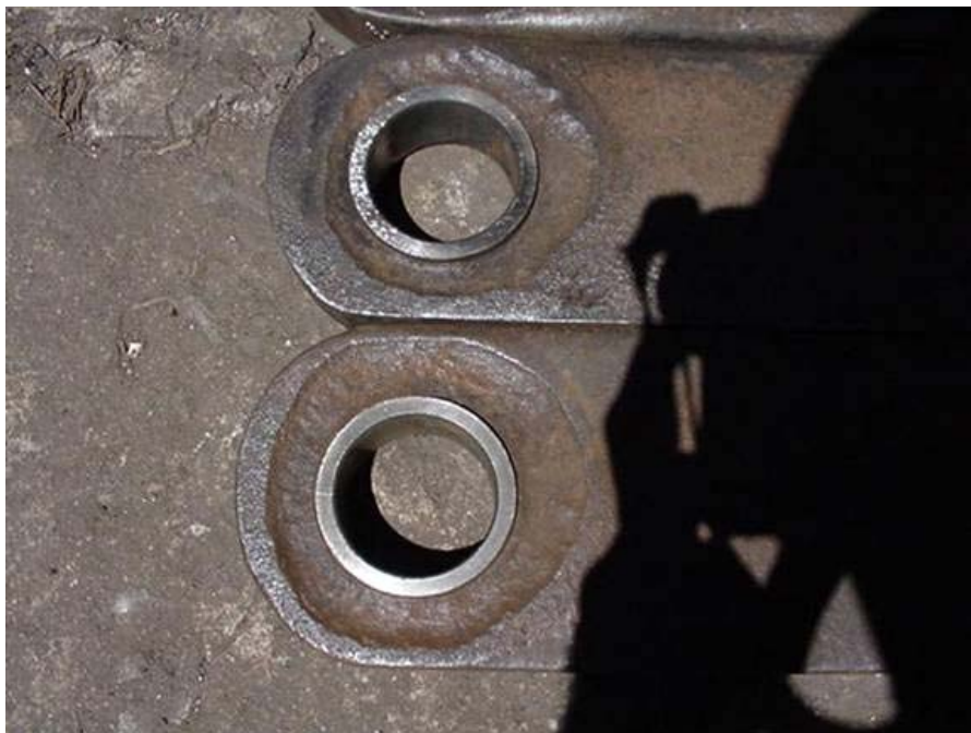
Figure 1. Worn Ausrex chain outer links.
