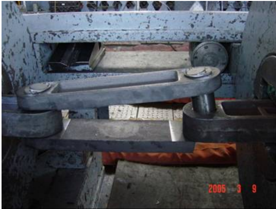
Figure 18. Failed new link 3 sample.
