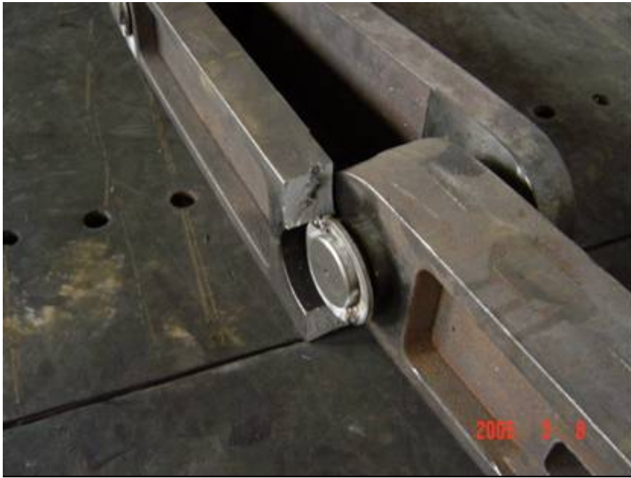
Figure 16. Failed defective new link 2 sample.
