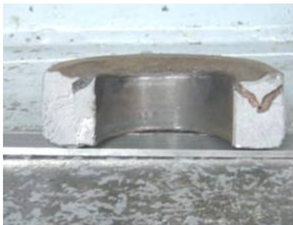
Figure 5. Failed section B1-B2-L1-L2.
