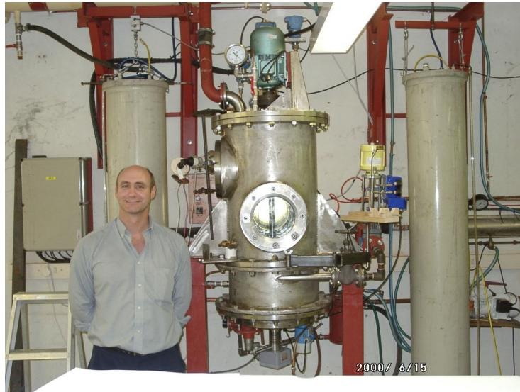
Figure 4. General view of pilot scale pan with vacuum condensate tanks on either side.
