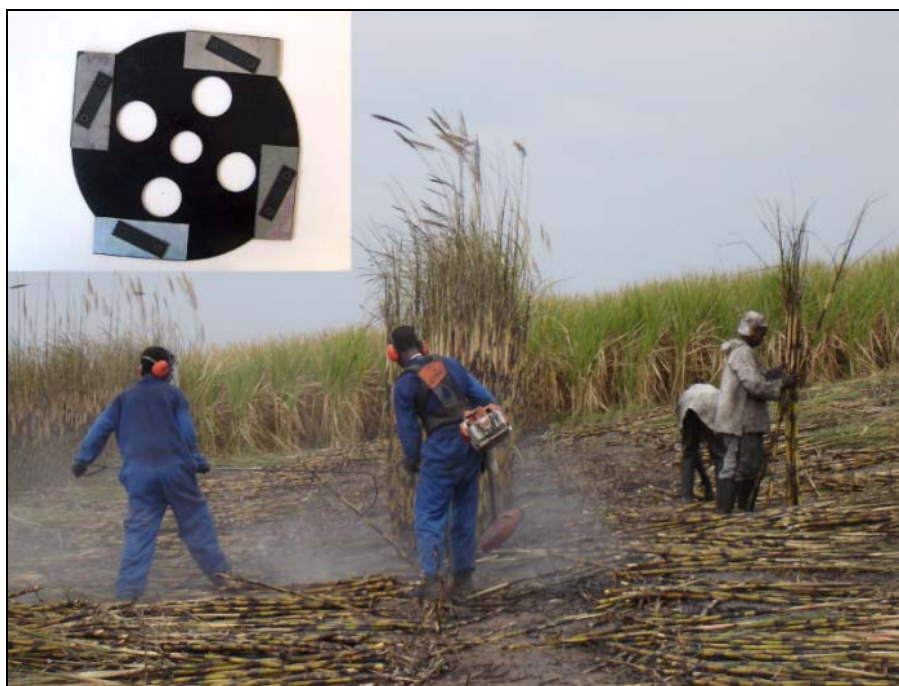
Figure 1. The Illovo mechanical cane cutter used in conjunction with a crook to pull cane into windrows. The insert illustrates the blade with replaceable edges.
