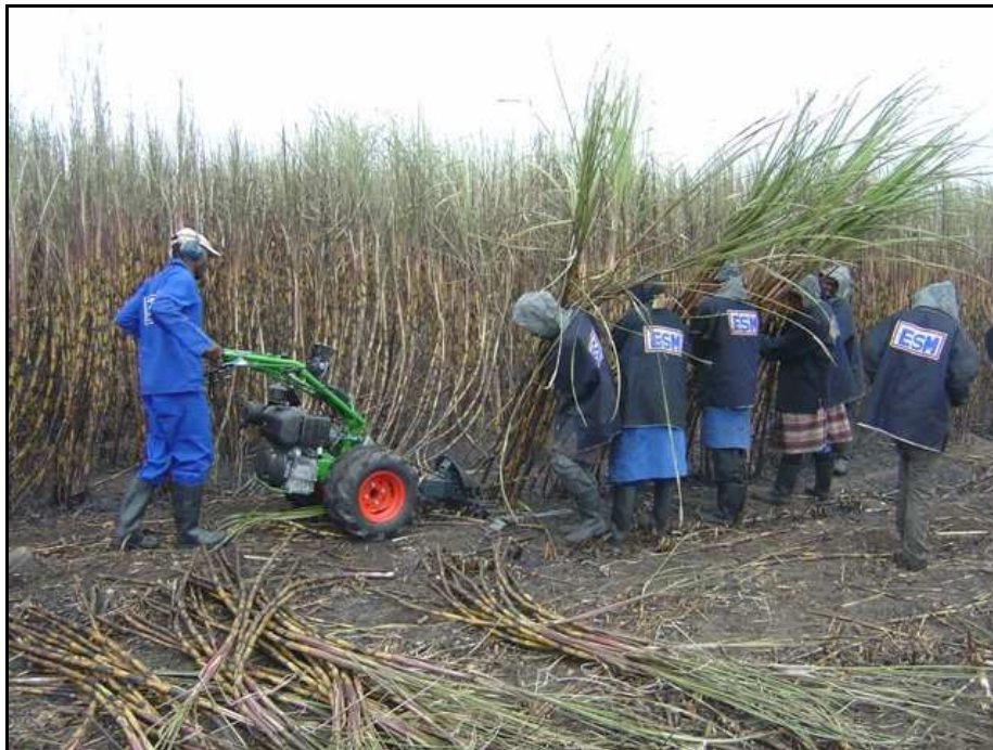
Figure 2. Operation of the CaneThumper®, showing the sorters pulling the cane forward in preparation for cutting.
