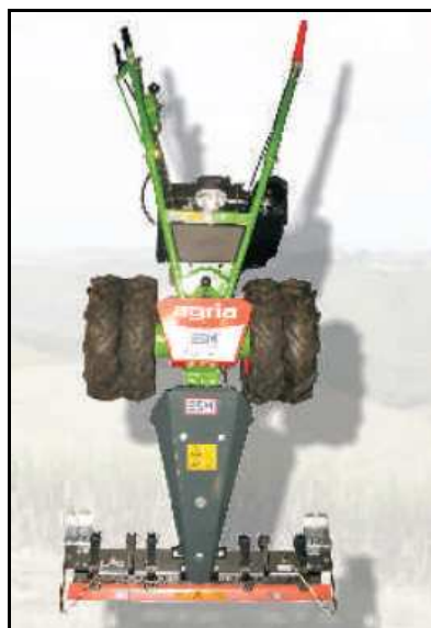
Figure 1. The CaneThumper ® with a single cylinder diesel engine and double action sickle bar cutter developed for harvesting sugarcane.
