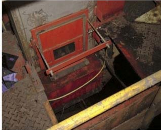
Figure 5. 'Trapdoor' in bottom of NIR chute with glass scanning window and mounting sill and bracket for scanhead box.
