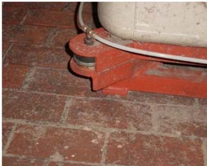
Figure 4. Two-part steel frame and air springs to reduce the effects of factory vibration on the NIR spectrometer.
