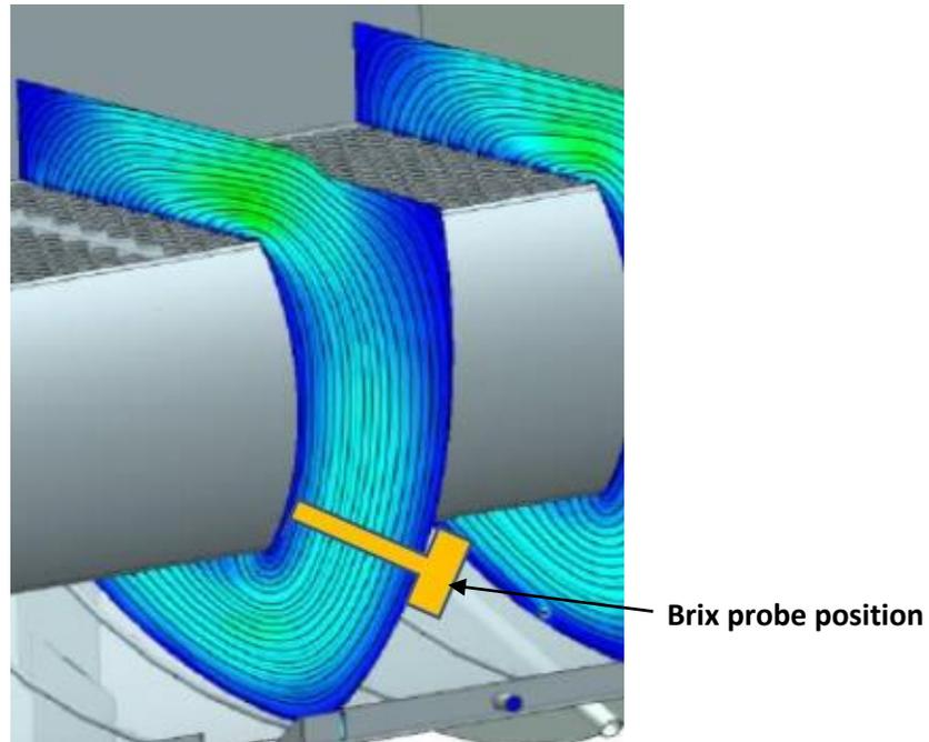
Figure 4. Transverse flow pattern in Bosch CVP.
