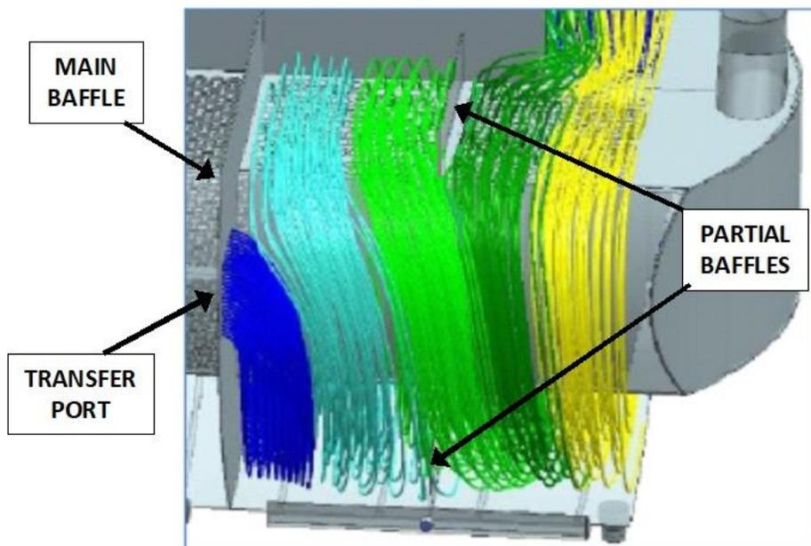
Figure 5. Arrangements that provide longitudinal plug flow in a Bosch CVP.
