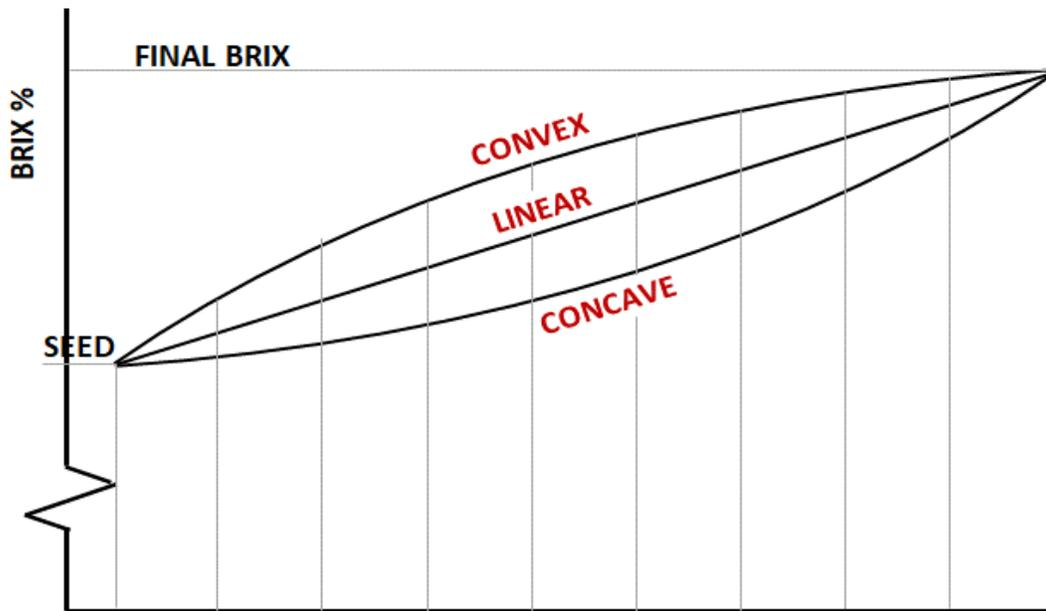
**Figure 2. Alternative Brix profiles for 10-compartment CVP.**
