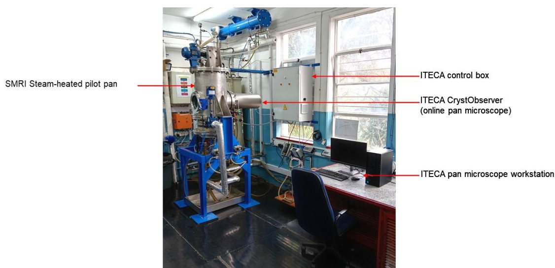
Figure 7. SMRI steam-heated pilot pan equipped with an online pan microscope
